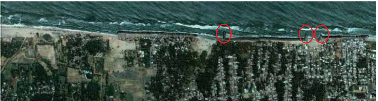
Figure 5.21: 17 th September 2005: first groynes built towards south.
