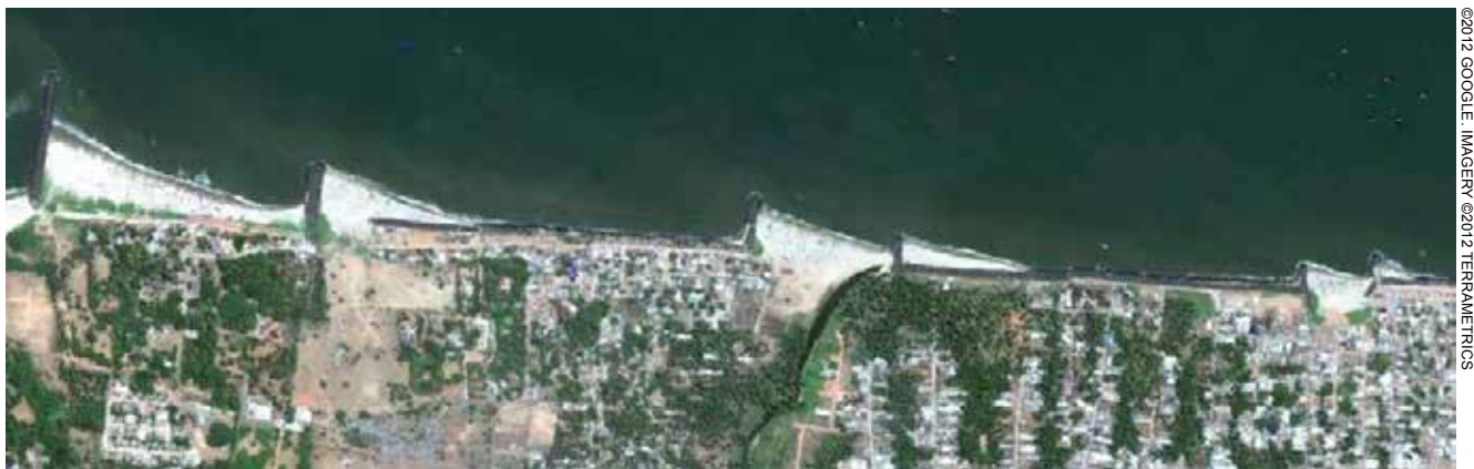
Figure 5.19: Series of 7 groynes built along Tamil Nadu coastline, north of Puducherry.
